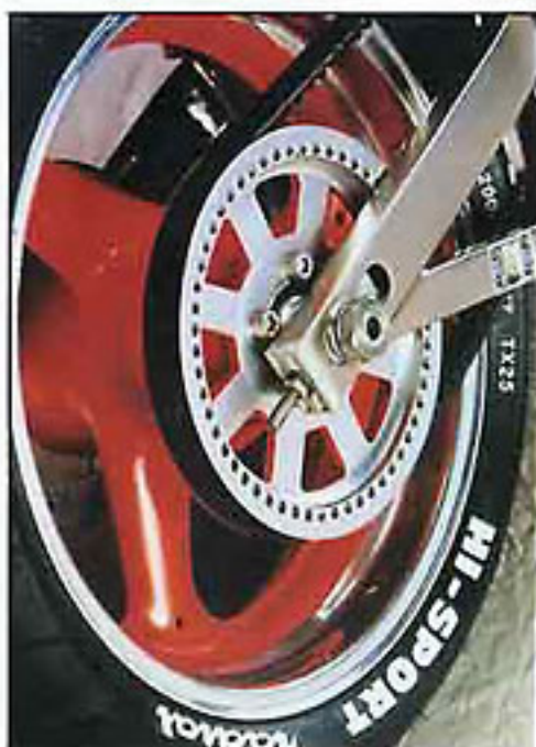
The standard Buell rear wheel has been widened and now measures 6.1x17".
