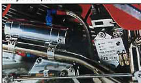
The Continuous Traction System (CTS) allows gear changing at full revs.
