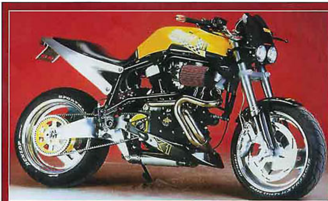
The standard Buell rear wheel has been widened and now measures 6.1x17".
