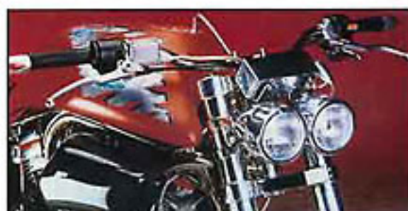
The front end features R&R twin headlights and triple trees.
