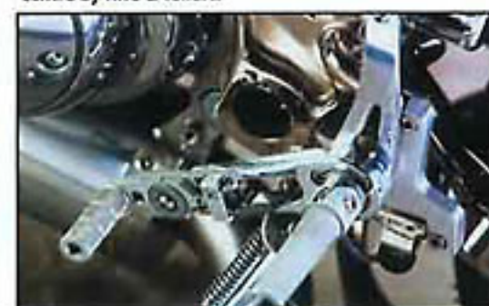
The adjustable rearsets are a combination of Buell passenger pegs and Tarazzo levers.
